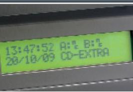
LCD with backlight shows recorder mode, time and date.
