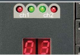
Dual LED level indicators for each recording channel.
