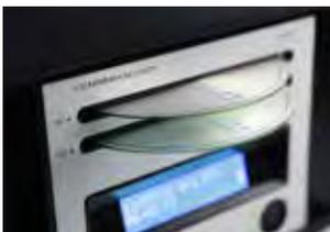
The **922IP Recorder** makes **two audio recordings** simultaneously. Producing two identical copies on two separate CDs. (In recorder sections CD A and CD B.)
